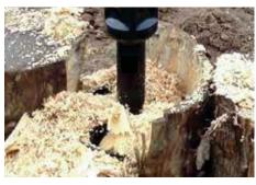
When the planer has achieved a deep cut, reposition to overlap the first hole and repeat the process until all of the stump is removed.
