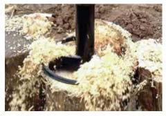
As the blades rotate they shave the wood into a tidy pile and pull the planer down further.
