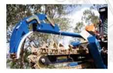
Our products incorporate many development features. The trench cleaner on our Trencher Attachments ensures a good clean cut with no residual spoil.
