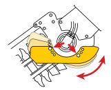
Adjustable Depth-control Skid allows for 3 different depth settings
