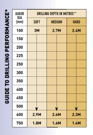
SKIDSTEER LOADERS LOW FLOW UP TO 65 HP S4 AUGERS 100mm-750mm Dia
