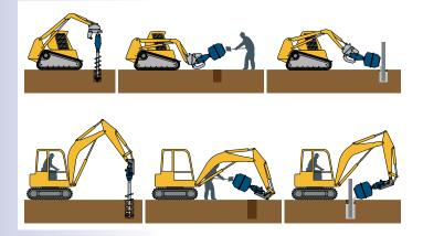
Ideal for fencing contractors, with the aid of the Mixer Cradle Hitch the Auger can be quickly removed and the Mixer Bowl attached and locked in place with the standard Auger Pin. After the concrete has been laid the Auger can be replaced for the next post.
