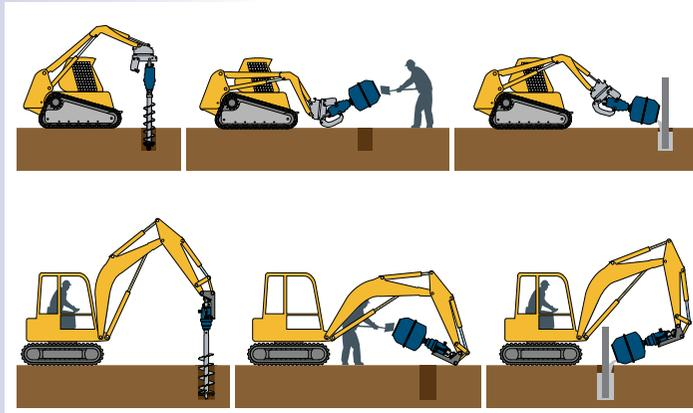
Ideal for fencing contractors, with the aid of the Mixer Cradle Hitch the Auger can be quickly removed and the Mixer Bowl attached and locked in place with the standard Auger Pin. After the concrete has been laid the Auger can be replaced for the next post.
